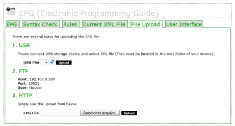
Figure 73 Loading Information for the XML File, via FTP or HTTP
